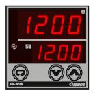
Press the setting key and the number of digits blinks. Press the UP/DOWN key to set the temperature and press the set key again to finish the setting.
