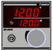
Press the setting dial and the number of digits blinks. Turn the dial to set the temperature and press the dial again to finish the setting.
