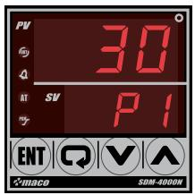
When the power is turned on, the current value is displayed on the PV window and the selected program pattern P1 is displayed on the SV window. Press the ENTER key for more than 2 seconds to execute program operation by pattern 1 to start. Use the UP / DOWN keys to select Pattern 2 (P2) or pattern connection control (P1P2) can be selected and operating. When it is set to the fixed mode, displays the PV / SV, such as the controller.
